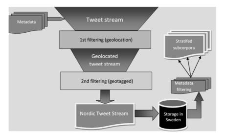
Figure 2: The pipeline for creating the NTS
