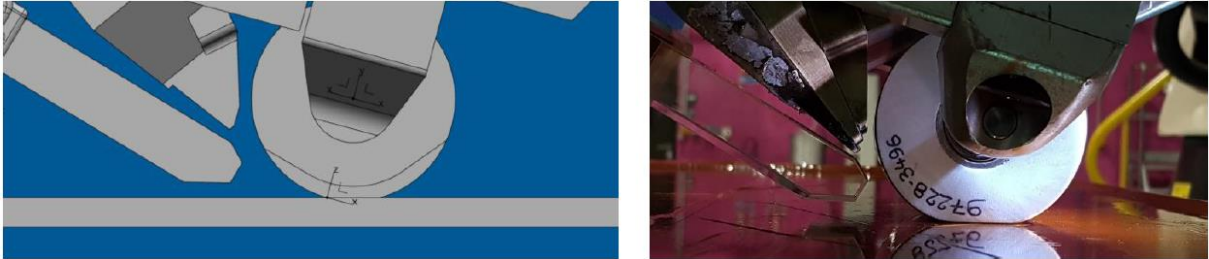
Figure 4 : Modelling flash lamp position according to actual fibre placement configuration
