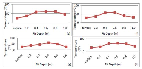
Figures 7: Variation of Temperature with Pit Depth for Pits (a) - (h) for the 8 pits.
