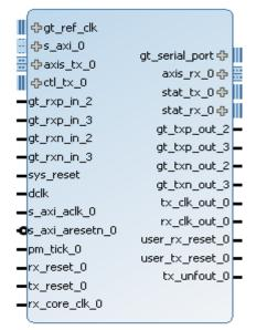
Fig. 2: System Design of VHDL based 40G EMAC
