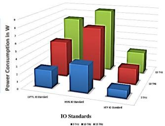
Fig. 7: Power analysis for VHDL based 40G EMAC
