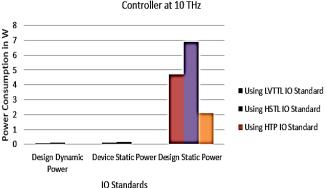
Power Consumption in W of vhdl based 40G Ethernet Media Access Controller at 10 THz
