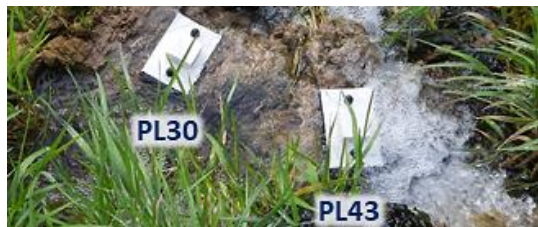
Figure 3. Limestone PLs installed near Roški waterfall.
