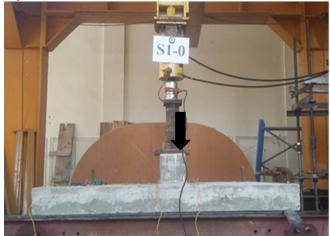
Fig. 2. Test Set-up for loading slabs.
