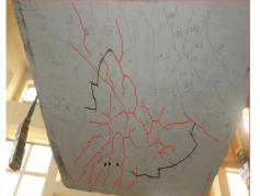
Fig. 9.Crack pattern and mode of failure S2-20.
