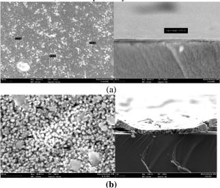
Fig. 1.Nanocrystalline thin film produced at the heating temperature 500 °C using (a) spin coating (b) chemical bath deposition method
