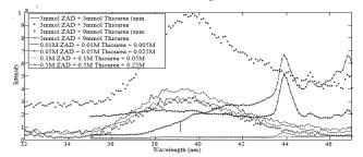
Fig. 3. Photoluminescence spectra of ZnS nanocrystals at different method, a ratio of Zn to S and concentration.
