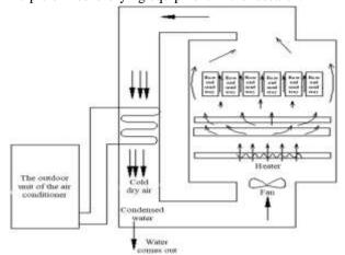
**Figure 1.** The schematic diagram of the operating principle of freeze-drying equipment
