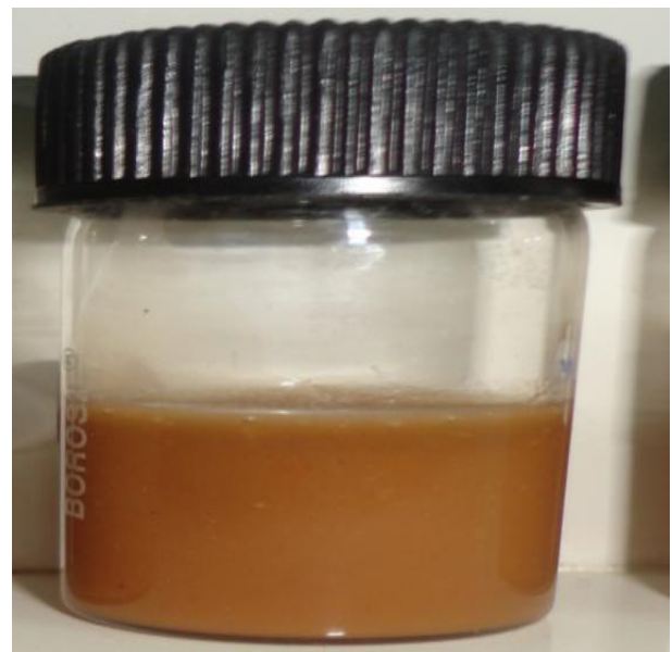
Picture 1. Photograph of the emulsion mud taken after 30 days of settling time.
