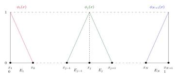
Fig 2. Piecewise smooth linear basis functions  $\varphi_1, \varphi_i, \varphi_{n+1}$  [13].
