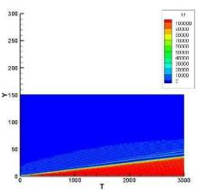
Fig 4. Acoustic wave propagation graph in one domain using the finite element method (T - time (s), Y - depth(m)).
