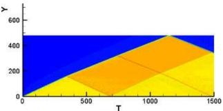
Fig 3. Acoustic wave propagation into three domains using the finite difference method (T - time (s), Y - depth(m)).
