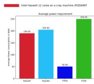
The big advantage of FPGAs: CPU and GPU have comparable energy requirements (200W vs 250W) whereas FPGAs require five times less.
