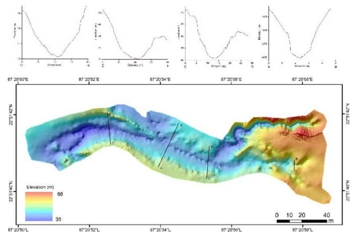
Figure 4. DEM of the total gully channel with some representative cross-sections. Lines AB, CD, EF, GH shows the location of the profiles.
