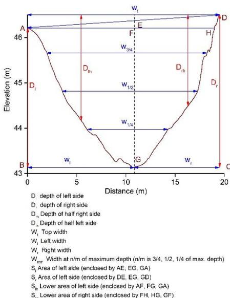
**Figure 6.** Morphometric parameters measured from a gully cross-section.
