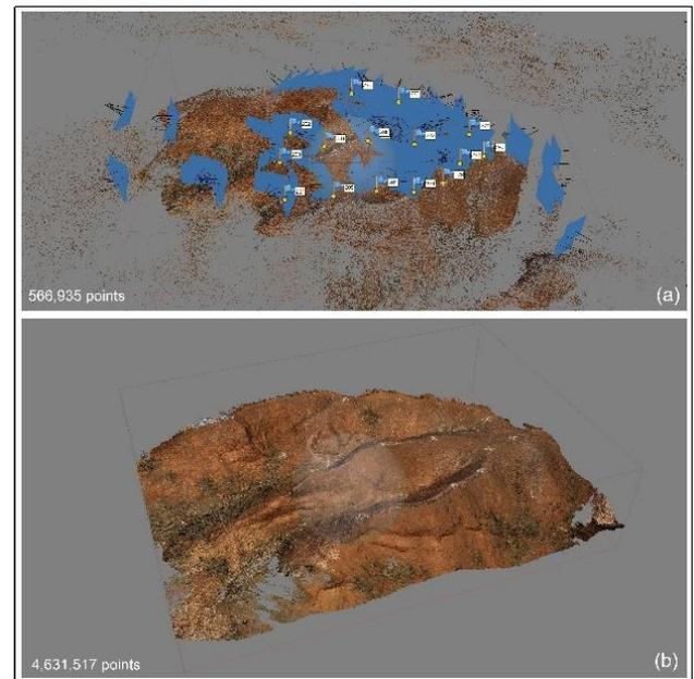
Figure 2. Perspective views of the gully head region (a) Sparse point cloud with location of cameras and GCPs marked (b) Dense point cloud.
