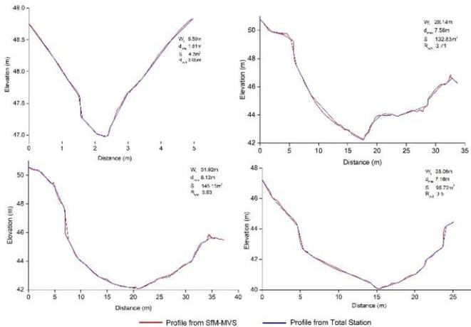
**Figure 5.** Cross-section comparisons between Total Station (TS) data and SFM-MVS derived DEM data for similar profiles along the gully channel.
