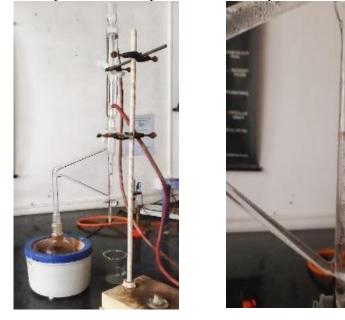
Figure no. 3: Volatile oil extraction performed by using Clevenger apparatus
