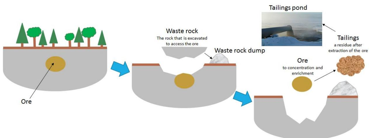
FIGURE 3. Waste generation in the mining process (reworked from SGU 2017).
