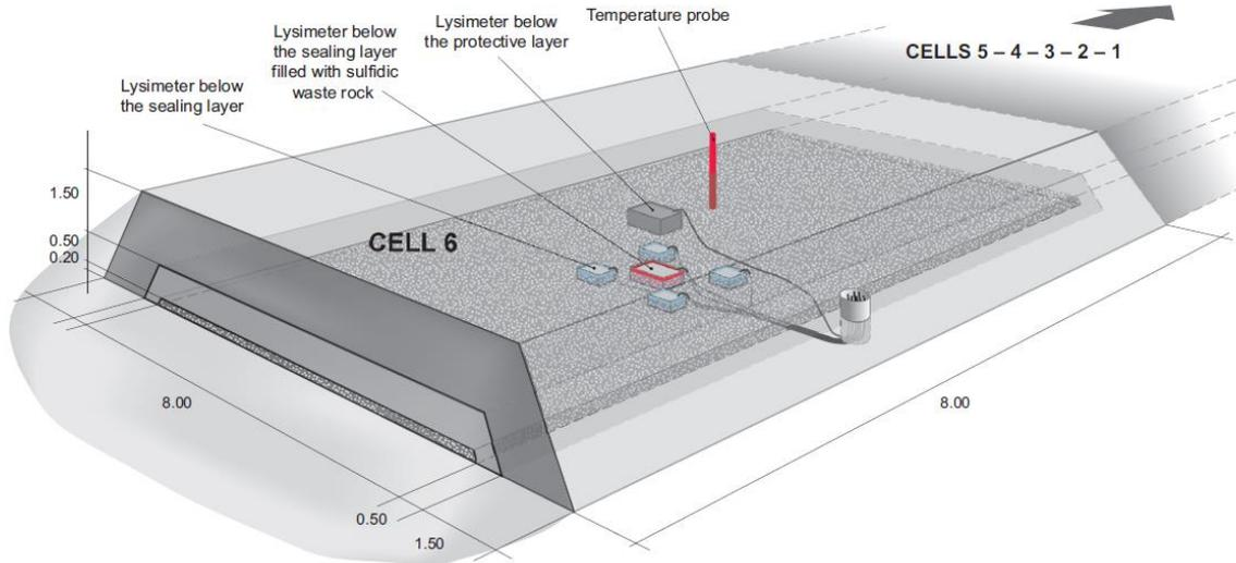
FIGURE 24. Sealing layer pilot technical performance monitoring.
