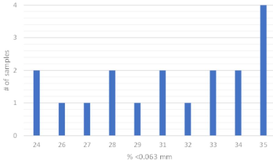
FIGURE 11. Variation in PSD (<0.063 mm) in till from the same till quarry.
