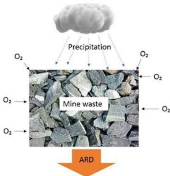
FIGURE 2. Descriptive figure of acid rock drainage (ARD).
