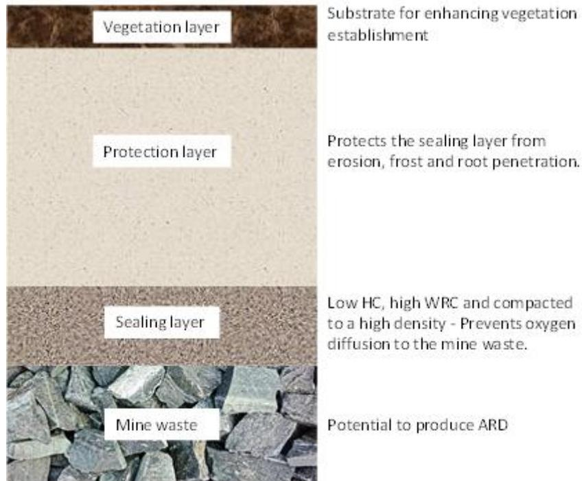
FIGURE 5. A describing figure of a typical soil “qualified” cover system in Sweden.
