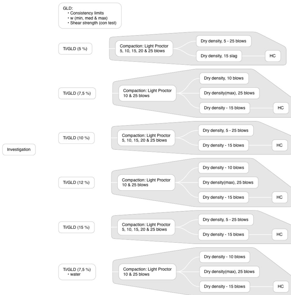
FIGURE 12. Example of scheme for elaboration of recipe of Ti/GLD mixture which meets the permeability requirements.
