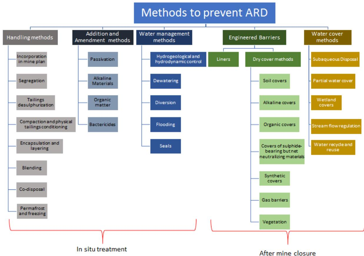
FIGURE 4. Different methods to prevent ARD from mine waste according to the GARD-guide (Verburg et al 2009).
