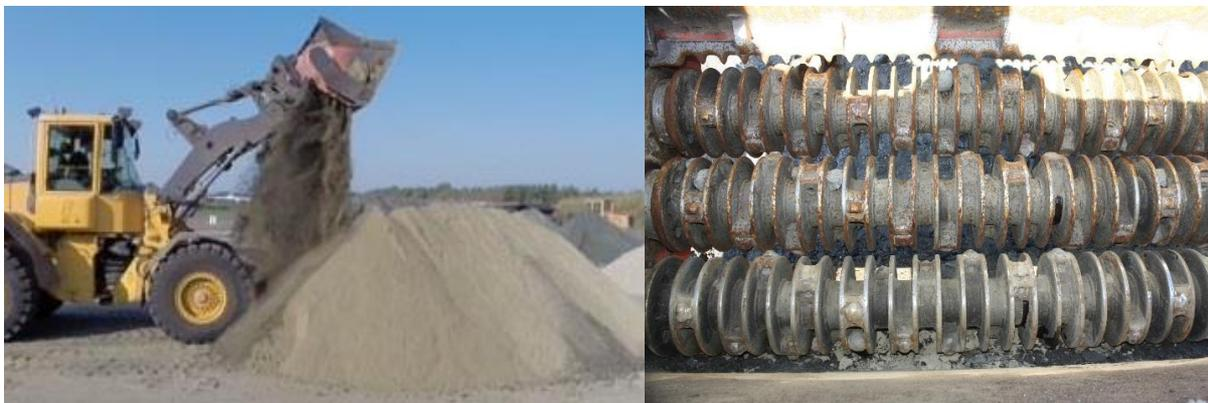
FIGURE 18. Bucket mixing by ALLU shovel (close up on the shovel).
