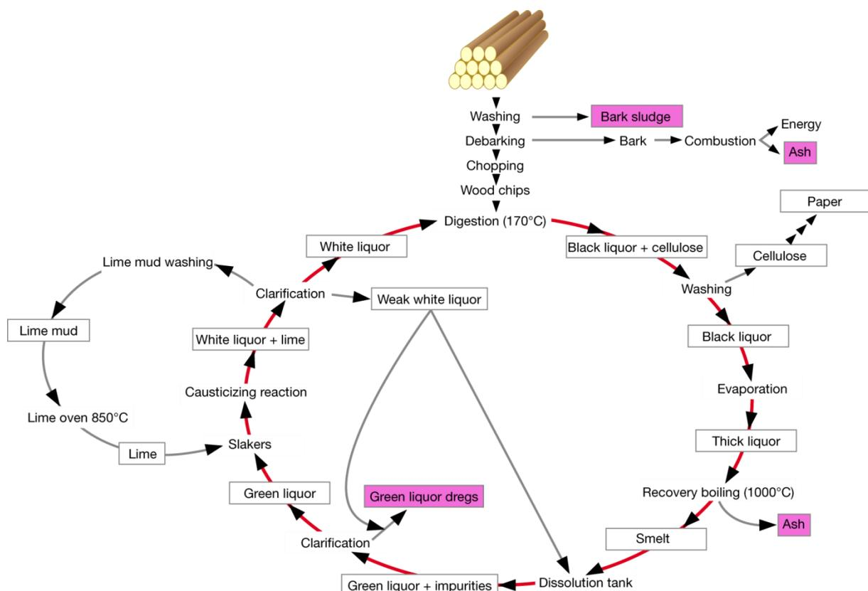
FIGURE 1. Retrieval of GLD from the sulfate process.
