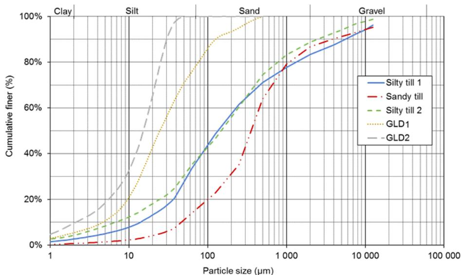
FIGURE 10. Examples of particle size distributions of various sieved tills (fraction  $< 20$  mm) and GLD from two different paper mills (Smurfit Kappa- and BillerudKorsnäs paper mill).
