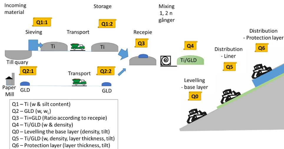
FIGURE 14. Conceptual model of the activities within the remediation process using Ti/GLD as sealing layer, where Q1-Q6 are quality control steps.
