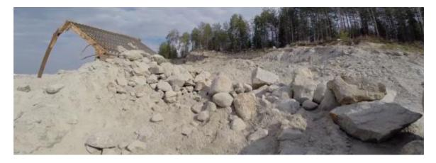
FIGURE 9. Till contains all particle sizes from fine soil to boulder, depending on the original bedrock and the glacial transport distance.
