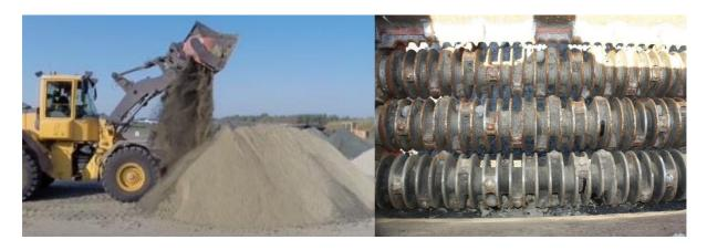
FIGURE 18. Bucket mixing by ALLU shovel (close up on the shovel).
