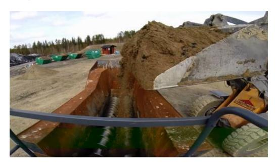
FIGURE 20. Loading a forced mixer with pre-mixed Ti/GLD.
