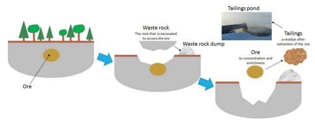
FIGURE 3. Waste generation in the mining process (reworked from SGU 2017).
