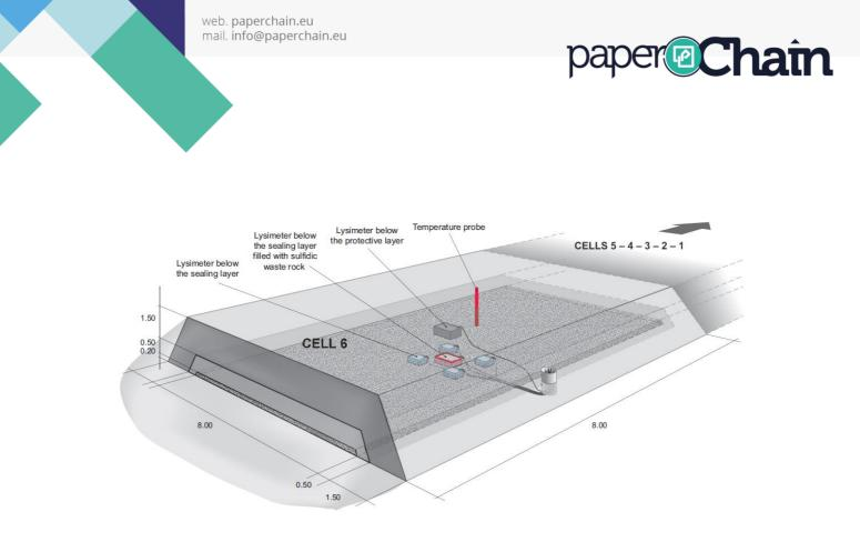
FIGURE 24. Sealing layer pilot technical performance monitoring.
