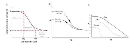
FIGURE 7. A) A typical SWCC, where  $\psi$ a is the air-entry suction,  $\psi$ r the water entry value,  $\Theta$ s the nearly saturated water content and  $\Theta$ r the residual water content (reworked from Tinjum et al 1997). B) A typical SWCC for desorption (drying) and sorption (wetting; reworked from Zhou et al 2012). C) A typical SWCC for clay, silt and sand (reworked from Sillers et al 2001).
