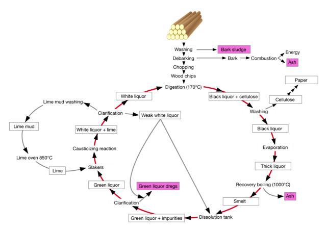
FIGURE 1. Retrieval of GLD from the sulfate process.
