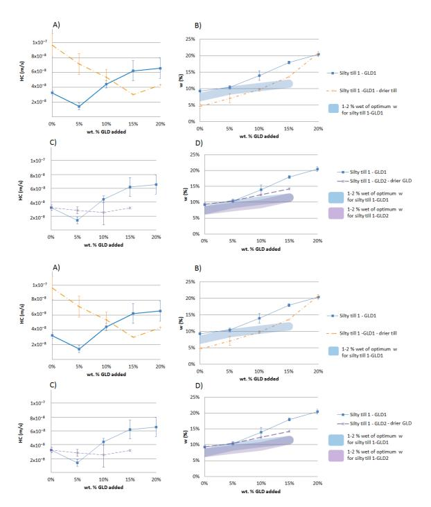
FIGURE 16. Hydraulic conductivity (HC) and molding water content (w) in different Ti/GLD mixtures.
