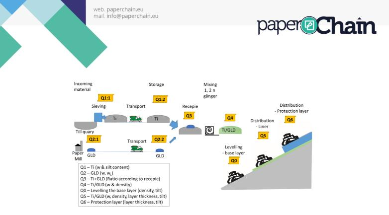
FIGURE 14. Conceptual model of the activities within the remediation process using Ti/GLD as sealing layer, where Q1-Q6 are quality control steps.
