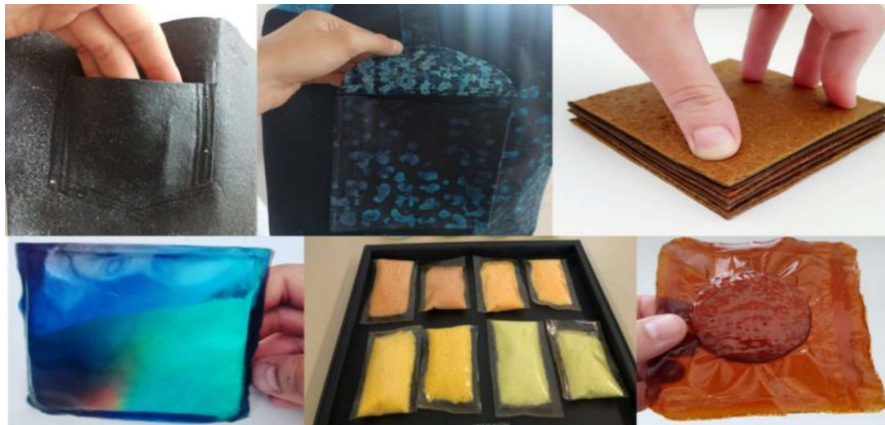
Figure 1: New generation of biopolymer-based material prototypes. Upper row illustrates new types of plant-based textiles made of discarded food waste. Bottom row depicts zero-waste and active film packaging intended for food and drinks.
