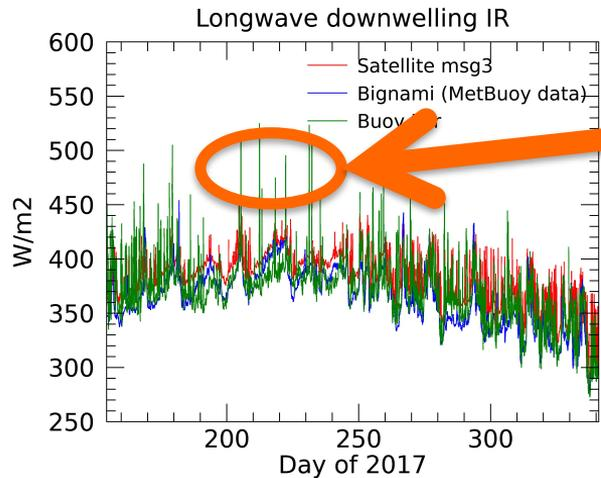
Small cloud passing in the field of view of the CGR4 Pyrgometer
