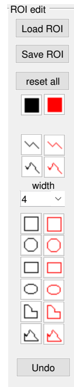
Figure 16.8: Manual editing controls
