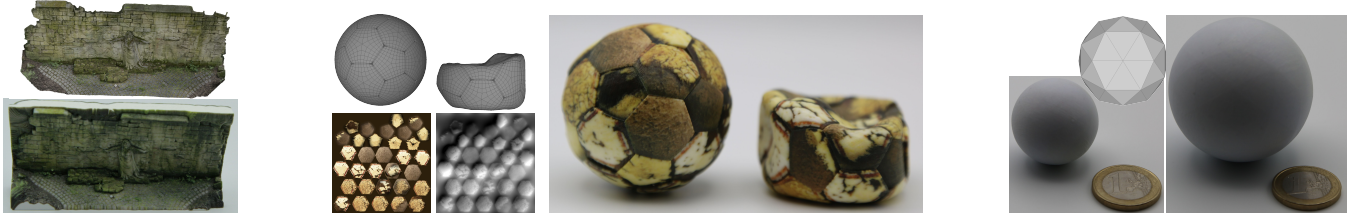
Fig. 1. Displaced signed distance fields provide an efficient way to address multiple challenges in additive manufacturing. Robust sign estimation allows 3D printing of open surfaces resulting directly from 3D scanning (left). Displaced signed distance fields allow the inclusion of meso-scale surface topography in the form of a displacement map (center) at virtually no extra cost, and the direct fabrication at device resolution of curved triangles (right). The same 80-primitive input (inset) allows the fabrication of a 3cm and a 5cm sphere without subdivision or further tessellation.
