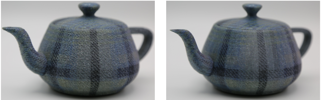
Fig. 15. A 13-cm teapot printed with a dishcloth displacement map (left) and without (right).
