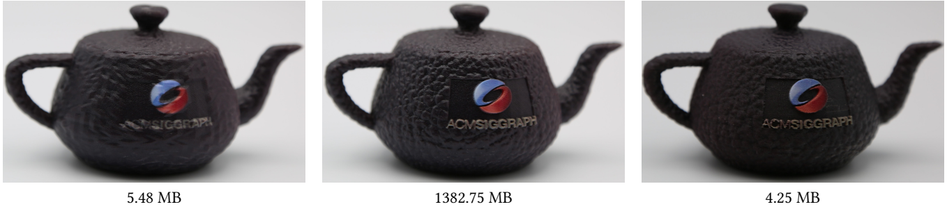
Fig. 14. A printed 9-cm teapot with 1 surface subdivision (left), 5 surface subdivisions (center), and displacement map applied using our method (right). Under each image we give the file size used to encode the geometry, including the displacement map for our method.
