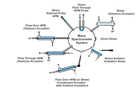
Figure 2-3: Membrane-introduction mass spectrometry (MIMS) interfacing configurations
