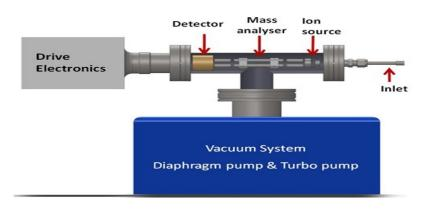
Figure 2-2: The classic components of a Membrane Inlet Mass Spectrometer (Courtesy of NTUA D5.1)
