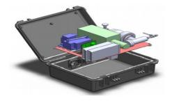
Figure 2-4: Portable RESCUE MIMS (Peli case) (Courtesy of NTUA D5.1)
