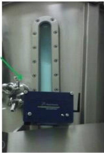
Spectral Probe NIR Analyzer installed on viewing window of Glatt FBD without any drying Modification
