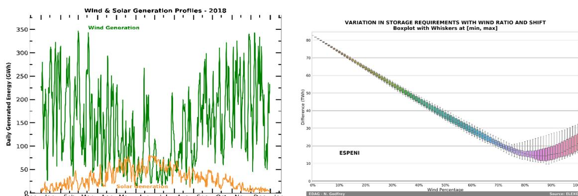
**Figure 5a** Wind and solar electricity production **Figure 5b** Wind and solar ratios – combined impact
