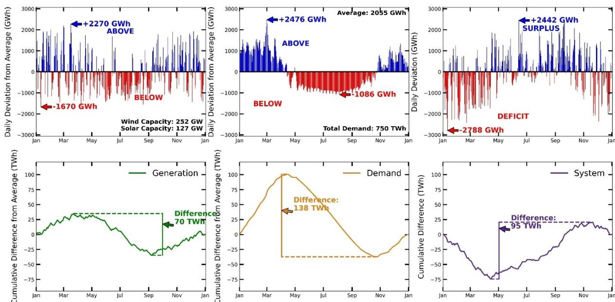
**Figure 10** Daily + cumulative **generation**, **demand** and **system** imbalance for electricity and heat (radiators)
