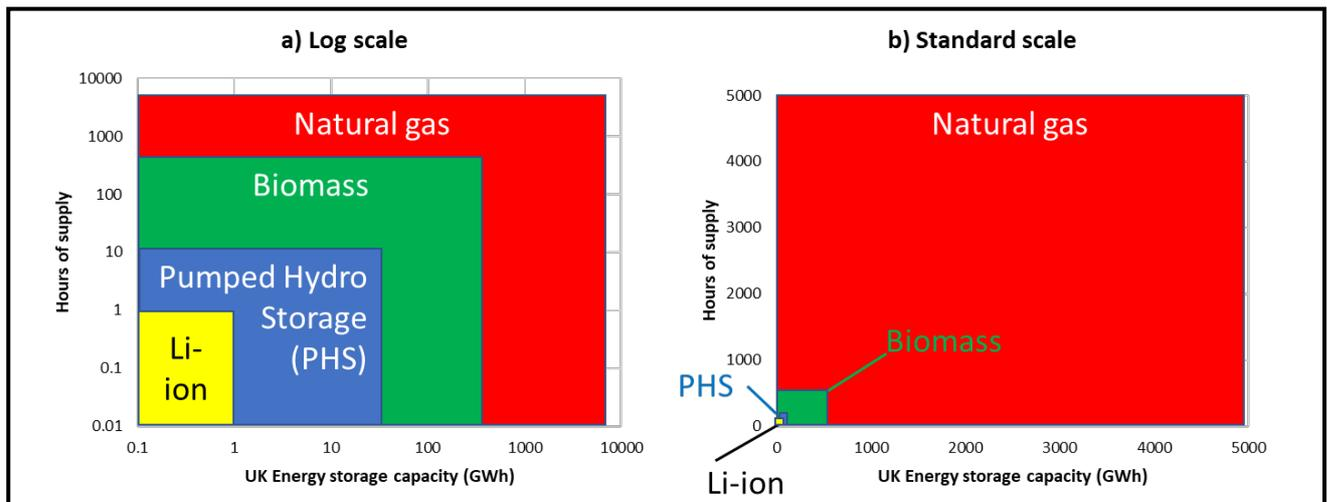
**Figure 13** Capacity and duration comparison **a)** log scale, **b)** standard scale
