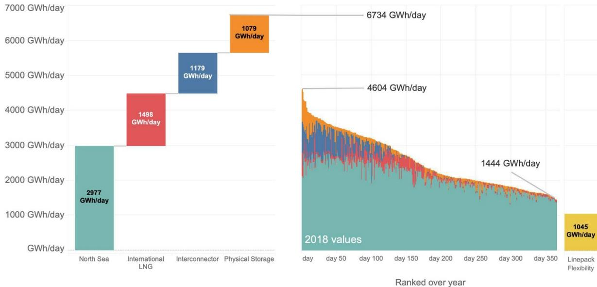
**Figure 1a** Daily gas storage capacities in GB **Figure 1b** Load-duration curve for gas supply in 2018
