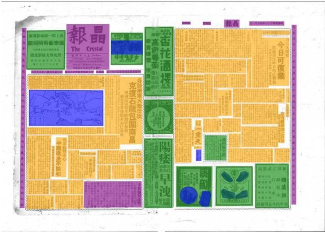
Fig. 2: The page fully manually annotated from our ground truth set (orange = article, blue = image, green = advertisement, purple = header and marginalia). Jing bao 晶報 (The Crystal), April 21, 1939, pages 1+4.
