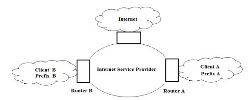
Figure 3 : Architectureusing the technique"NetworkIngress Filtering".
