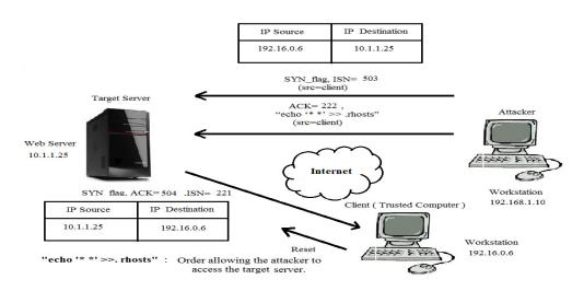
Figure 2 : Stages of the IP Spoofing attack.
