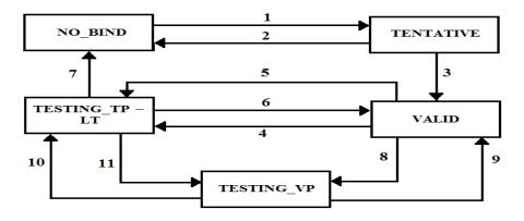
Figure 8: The finite state machine of the FCFS SAVI method.
