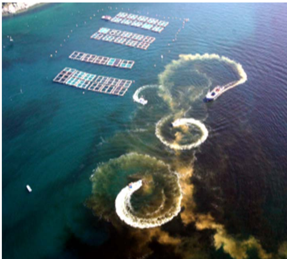
Fig. 1. Aerial view of merry-go-round clay dispersal off Yokjido Is on south coast of Korea, to control fish-killing Cochlodinium bloom approaching fish cages, August 21, 2008, photographed by Jong-Suk Jung. Source : Hak Gyoon Kim, Pukyong National University, hgkim@nfrdi.go.kr
