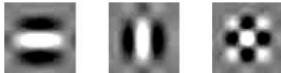
Fig.1. H,V,D bands from 2-D DWT basis obtained using Daubechies filter(length-14)
