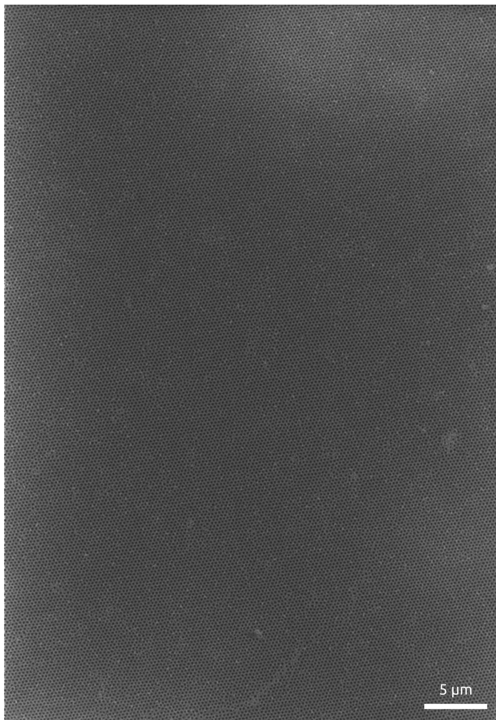
Figure S8: Top view SEM micrograph of a nanoporous single domain array over an area of  $60 \times 41 \mu\text{m}$ .
