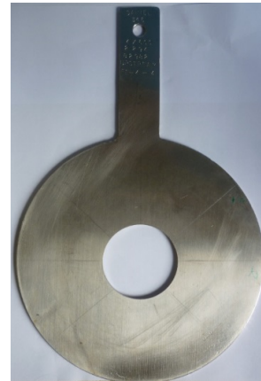
Figure E4.2.3: An EEC orifice plate
