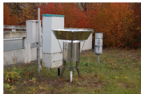
(b) Weighing gauge installed in field
