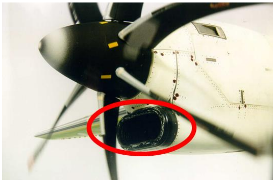
Figure 2: Engine Air Intake. Top: EAI of a turbo-propeller engine. Bottom: the five zones of the surface to protect of the EAI
