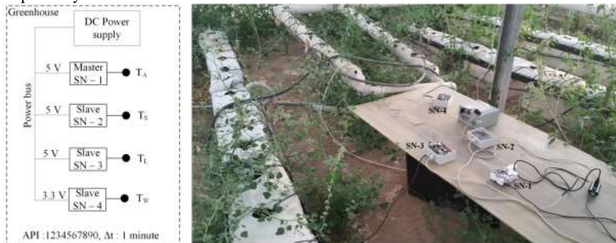
Figure 3 (a) Positions of sensor nodes in greenhouse, (b) Greenhouse experiments
