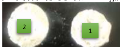
Figure 5: comparison of the clots formed from pasteurized milk using infrared radiation (1) and Classic method (2) at 72° C for 15 seconds.
