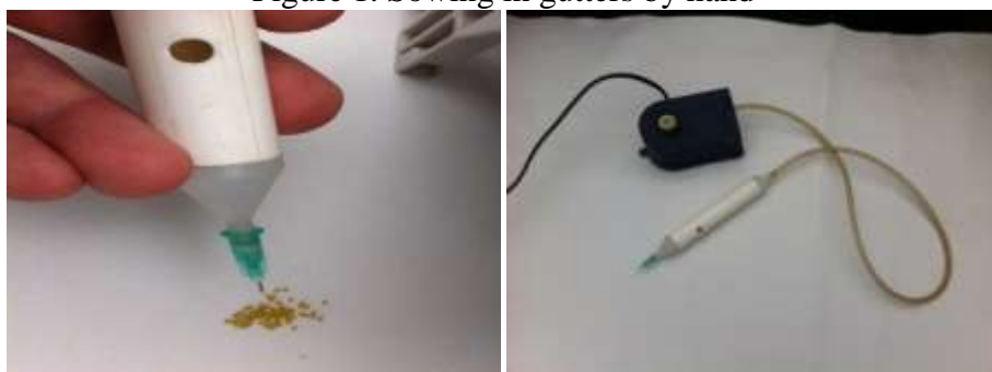
Figure 2. First equipment for seed drilling with seed
