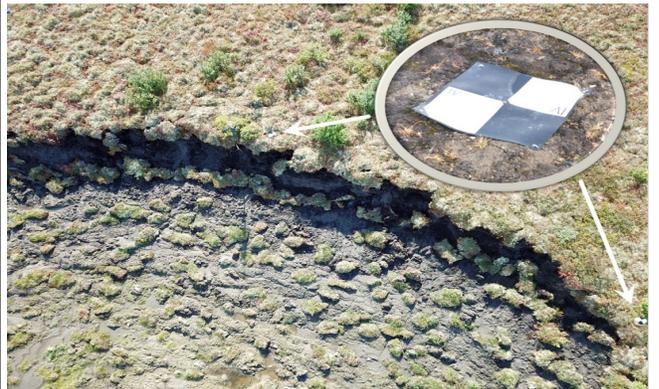
Figure 5: Ground control points (40 x 40 cm black/white rubber mat) around a thaw slump.
