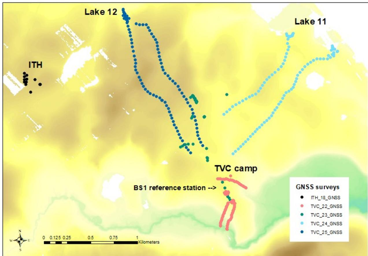
Figure 1: Overview of the measurement area, transects and grids around Trail Valley Creek (TVC).
