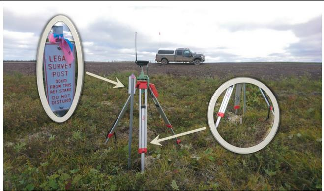
Figure 3: Reference station GS16 installed over a known point, close to the highway
