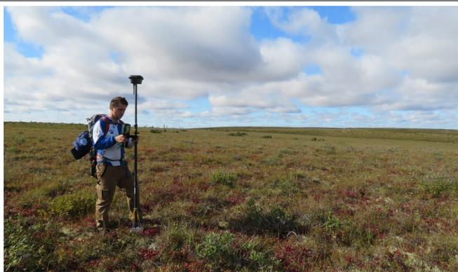
Figure 2: GNSS RTK-Measurements in field
