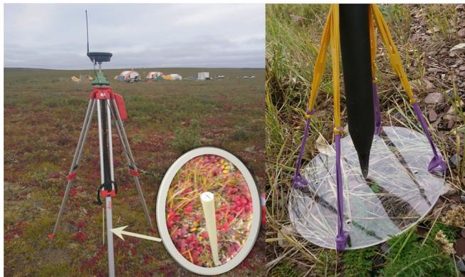
Figure 4: left: reference station close to Trail Valley Creek installed over stick, which was installed in 2016, right: Rover pole with 20 cm diameter PVC-plate
