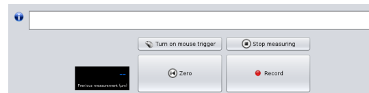
Figure 2.2: Measuring control panel. The number of digital displays will vary between 1 and 3 depending on what type of measuring platform hardware you have.
