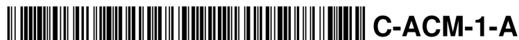
Figure 10.1: An example of a sample barcode produced by Tellervo for the Cornell lab. Note the label also includes the human readable code for the sample.
