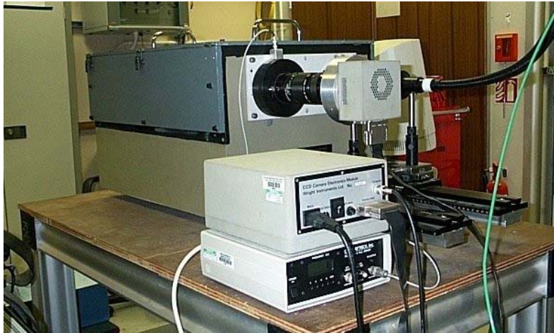
(a) The black trunking on the right contains the optical fibres from the tokamak. At the spectrometer exit, the grey lead carries the control signal for the FLC shutter. Connected to the shutter mount are the exit lenses and then the CCD camera. The two grey boxes in the foreground are the camera power supply (top) and the control system for the FLC shutter (bottom).
