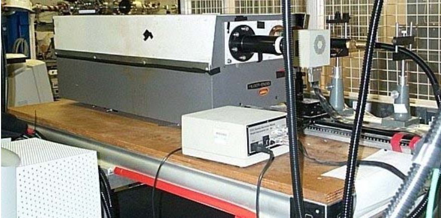
Figure 3.5: The CELESTE spectrometer - a 1m Czerny-Turner device fitted with a 1200\text{mm}^{-1} grating.
