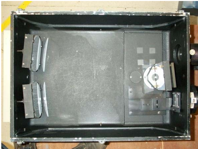
(b) Plan view with the lid removed showing the two spherical mirrors (left) and the grating (right).
