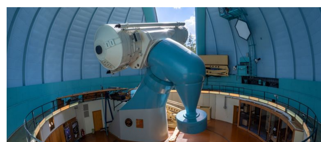
Figure 4. The 2-m Perek telescope in Ondřejov, Czech Republic (left panel). The right-hand panel shows a part of the normalized spectrum of TIC 235709086 around the Mg triplet.
