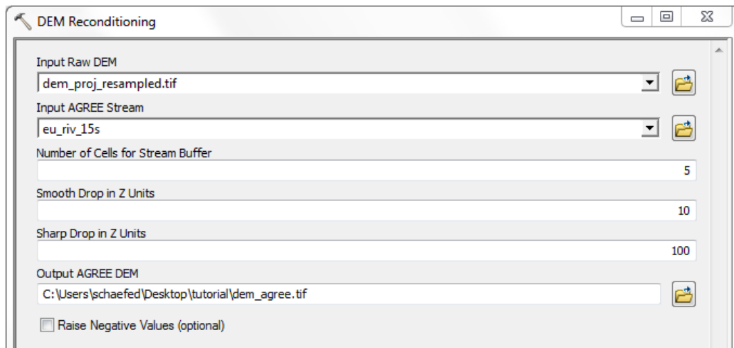
Figure 3.11: System Toolboxes -> Arc Hydro Tools -> Terrain Preprocessing -> DEM Reconditioning
