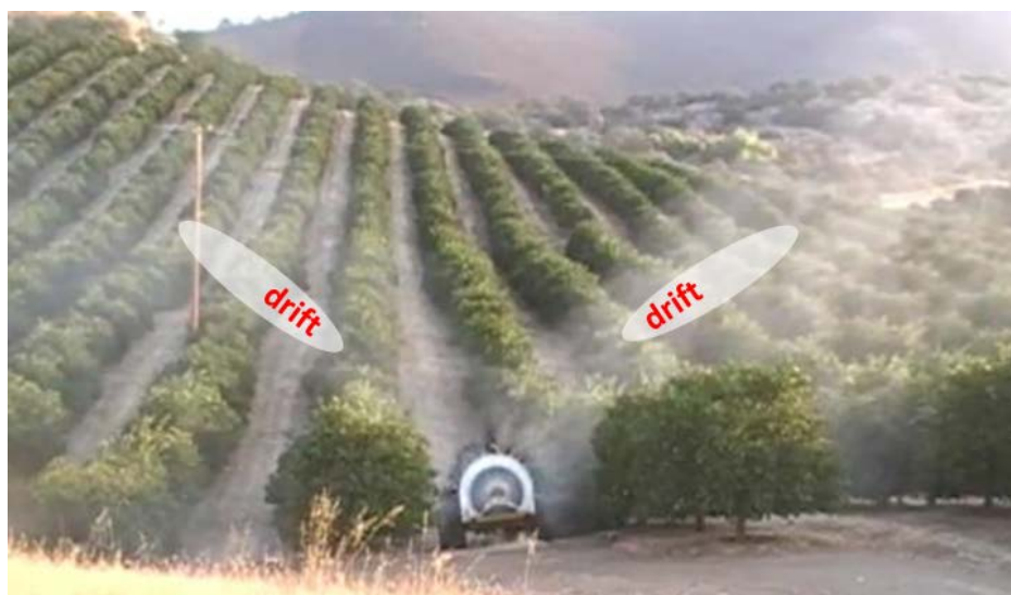
Fig. 1. Drift caused by conventional airblast sprayer in an orange orchard.
