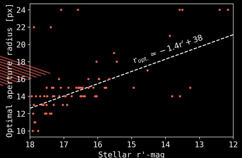
We perform aperture photometry on the dense starfield surrounding the hot Jupiter host Kepler-76. We find that the aperture radius should be optimized for the target's magnitude to achieve a lower RMS. This observation used 3x binning and 30s exposure times with the r' filter.
