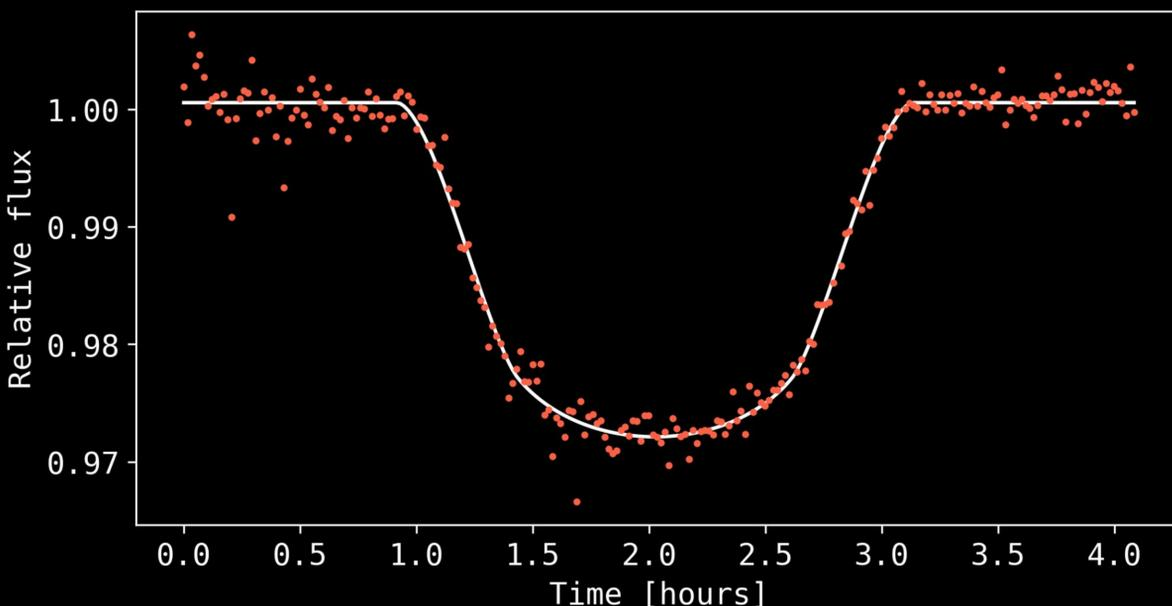
An r'-band transit of the exciting inflated hot-Saturn NGTS-5 b ( $r' = 13.5$ ). A fortuitous bright nearby reference star enabled a systematics-free photometric light curve. We use a nested sampler to fit the planet's radius, orbital inclination, and time of transit, along with a scalar vertical offset. We find that this single transit improves upon the discovery paper's system constraints (Eigmüller et al., 2019).
