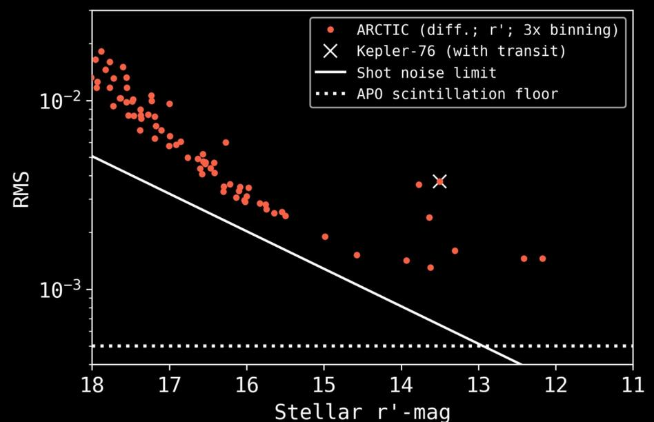
The unbinned magnitude-RMS relation for a single night of observations with 30s exposure times. Stars brighter than 15th magnitude routinely achieve near-mmagnitude precision. The shot noise limit and APO's scintillation noise floor are shown. Brighter stars deviate from the shot noise trend due to red-noise systematics, which can be largely detrended given a reference star of similar color and magnitude.
