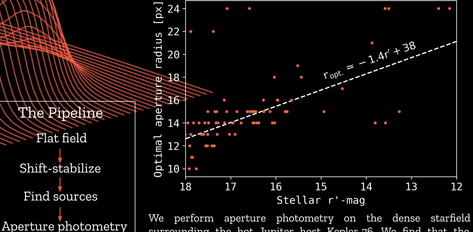
surrounding the hot Jupiter host Kepler-76. We find that the aperture radius should be optimized for the target's magnitude to achieve a lower RMS. This observation used 3x binning and 30s exposure times with the r' filter.
