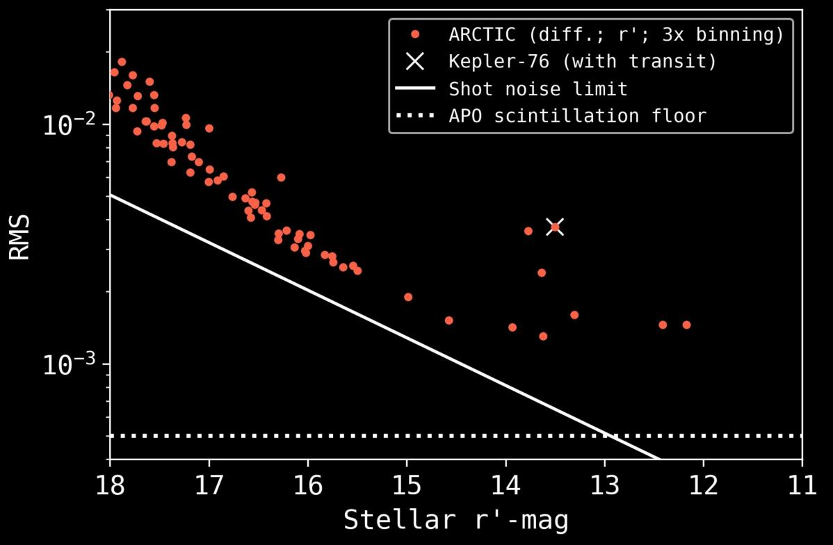
The unbinned magnitude-RMS relation for a single night of observations with 30s exposure times. Stars brighter than 15th magnitude routinely achieve near-mmag precision. The shot noise limit and APO's scintillation noise floor are shown. Brighter stars deviate from the shot noise trend due to red-noise systematics, which can be largely detrended given a reference star of similar color and magnitude.
