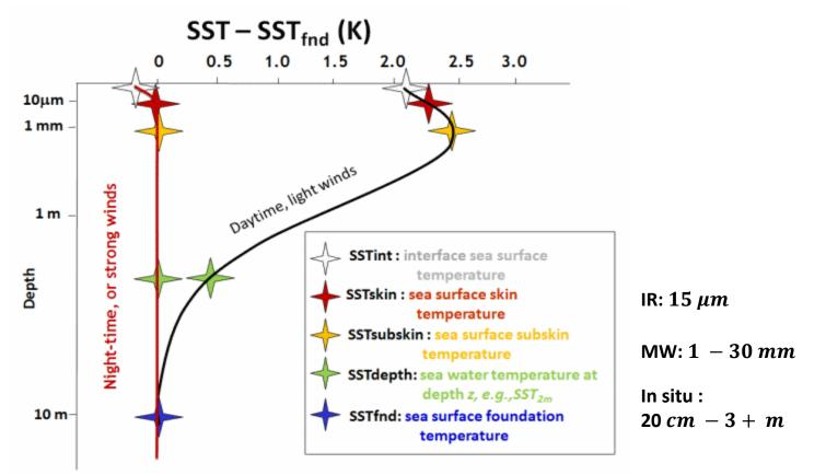
Hypothetical vertical profiles of temperature for the upper 10m of the ocean surface in high wind speed conditions or during the **night** (red) and for low wind speed during the **day** (black).
