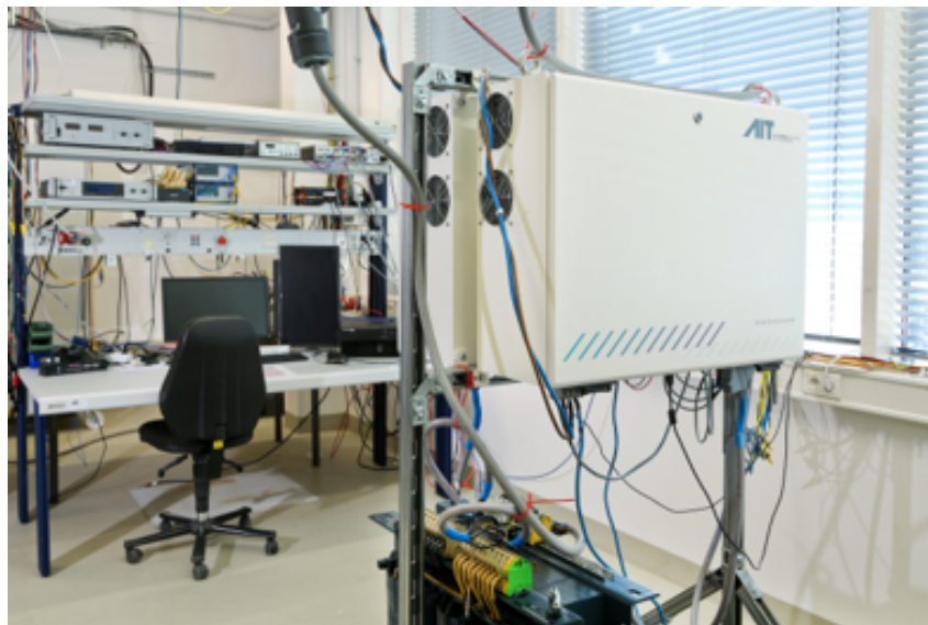
Figure 11: Laboratory setup with two AIT Smart Grid Converters in a back to back setup.
