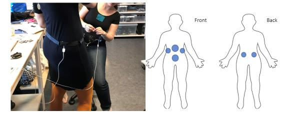
Figure 3: Left: One of the authors trying the hacked strain sensor belt. Right: Areas of interest for strain sensor.
