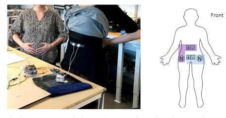
Figure 4: Left: The EMG sensor stitched on conductive textile panels. Right: Areas of interest for EMG sensor.
