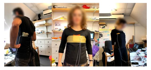
Figure 7: Wearing the Breathing Shell and testing the somatic impact of non-habitual breathing, through the shape-change sensor-actuator pillows. The tubes lead to the areas where the pillows are placed.
