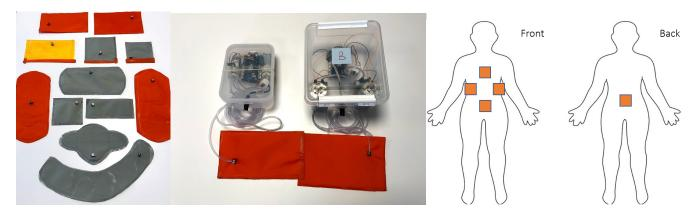
Figure 5: Left: Inflatable pillows. Center: Shape-change sensor-actuators. Right: Areas of interest for shape-change pillows
