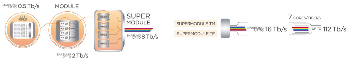
Fig. 1. Multi-Tb/s S-BVT transmitter based on VCSEL integration with modular approach.
