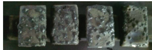
Fig. 11. Coated specimens after corrosion testing
