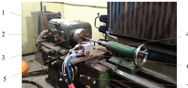
Fig. 1. Experimental stand for surfacing metal powders: 1 – lathe; 2 – movable machine carriage; 3 – three-jaw chuck; 4 – tailstock; 5 – machining part; 6 – plasmatron; 7 – control levers
