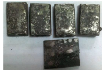
Fig. 12. Samples with cleaned surface from traces of corrosion
