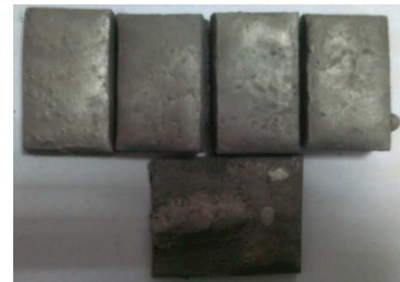
Fig. 10. Coated specimens prior to corrosion testing
