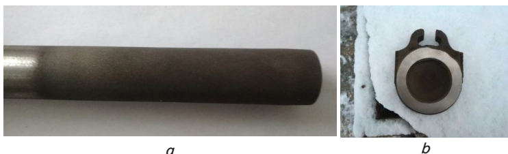
Fig. 2. Obtained parts during processing on the plasmatron: a – on a cylindrical surface; b – on a flat surface
