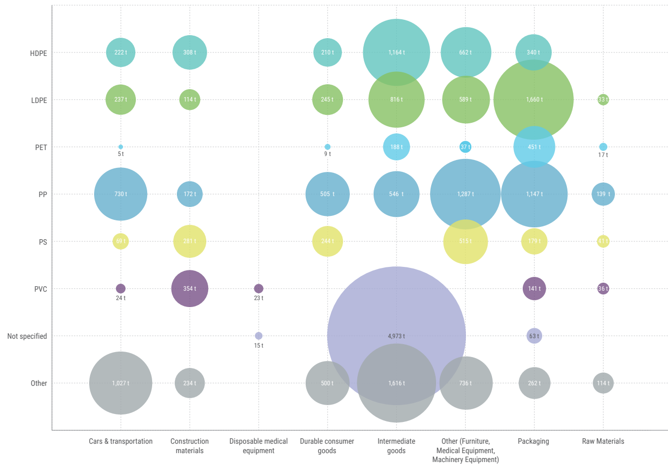
Figure 25: Polymer composition of different product applications used in Vejle
