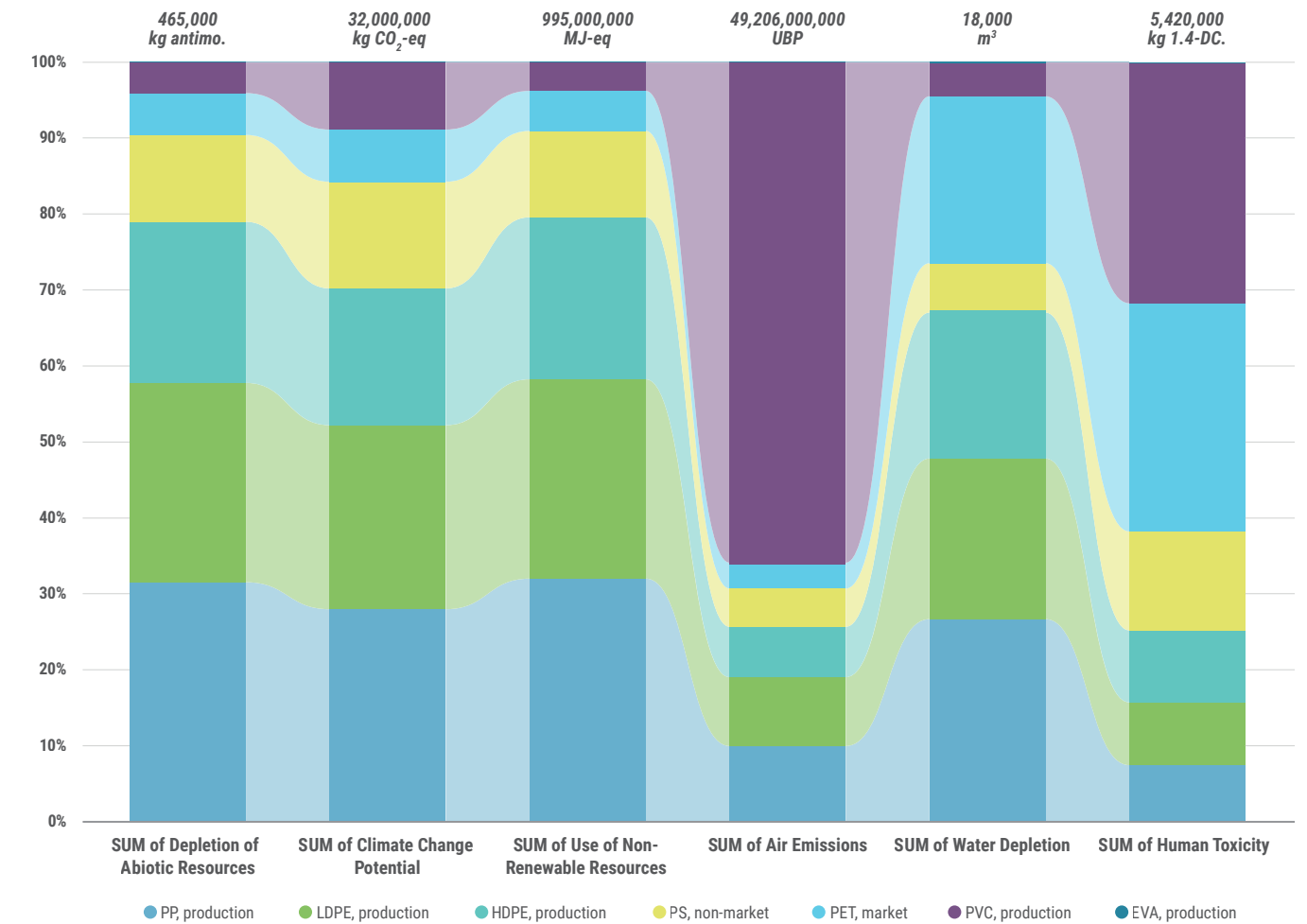
Figure 24: Relative contribution of different polymers to different environmental impact categories associated with the production of key polymers. 97
