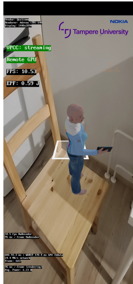
Fig. 7: Screenshot of the AR application used to measure the effect of offloading heavy computation. A streamed animated point cloud of a person holding a small tablet device is displayed in augmented reality on top of a real-world chair.
