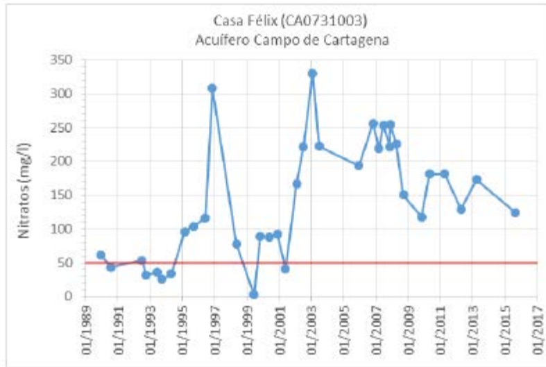
Figure 18. Nitrate concentration at borehole CA0731003 in groundwater body “Campo de Cartagena”.
