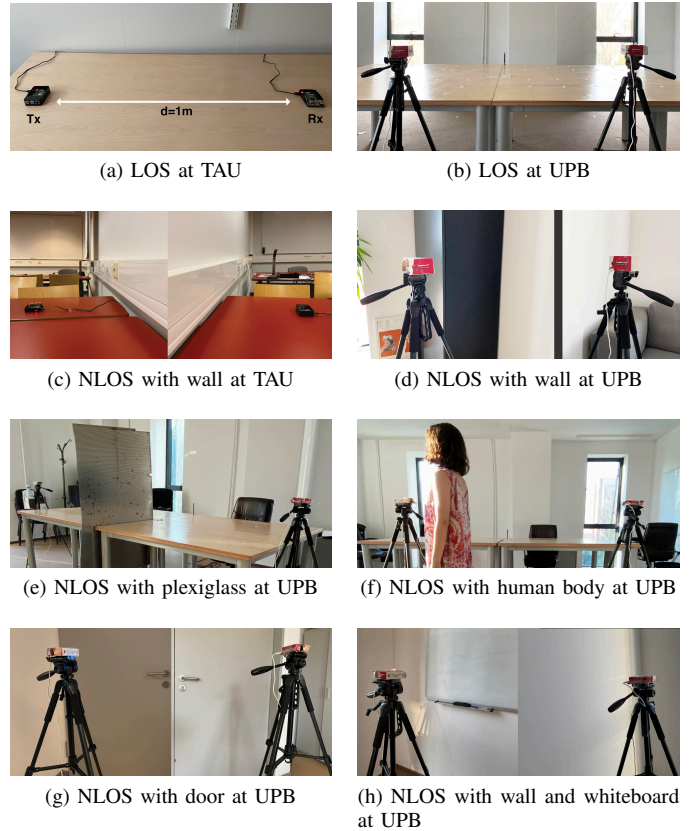
Fig. 4. The pictures of the receiver and transmitter in LOS and NLOS with wall acquired at UPB and TAU (Fig. 4a to 4d). Fig. 4e to 4h show NLOS scenarios with a plexiglass panel, human body, a door, and a wall with a whiteboard at UPB.
