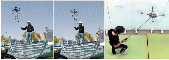
Fig. 8. AEROM providing a tool (left) and guiding a human (right).
