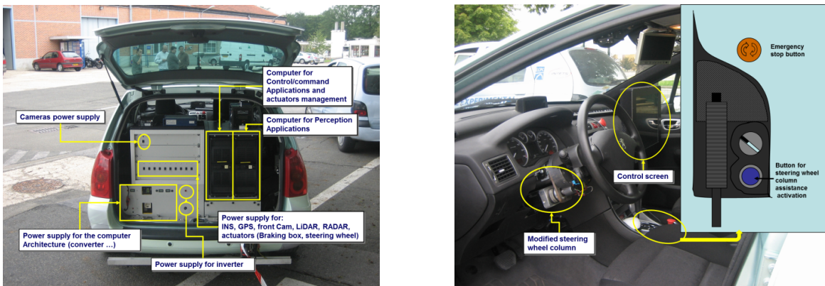
Figure 12. A dedicated real prototype for highly automated driving applications.
