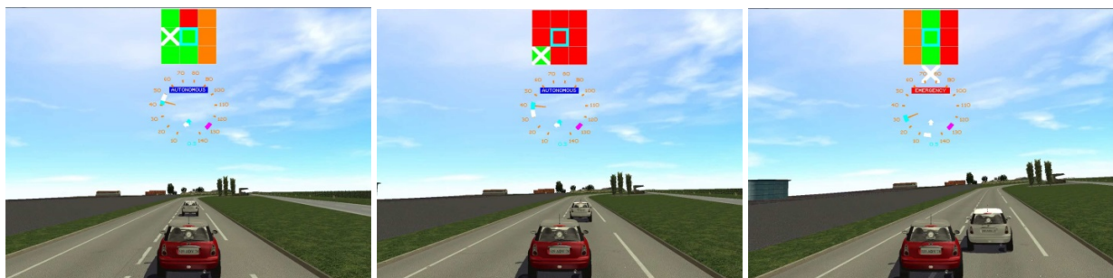
(a) the leader suddenly stops (left), the ego-vehicle starts changing lanes in autonomous mode (middle) but has to switch to emergency mode to avoid collision (right)
