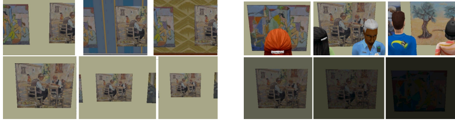
Fig. 2. Samples showing examples of different conditions simulated in the virtual environment. Row 1 (left) shows the simulation of different wall textures, row 1 (right) the introduction of virtual visitors, row 2 (left) changes in camera orientation and row 2 (right) changes in ambient lighting.
